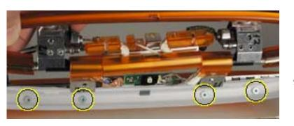
8. Remove the four exterior screws on the display housing.
