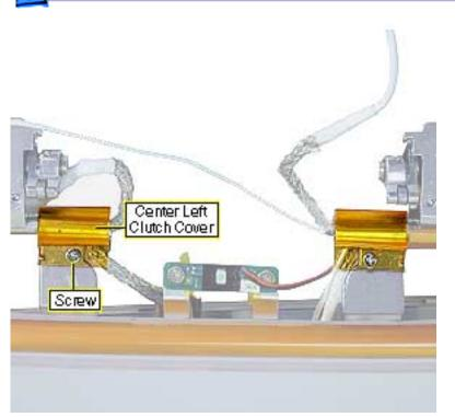
6. Remove the screw on the back of the center left clutch cover.
