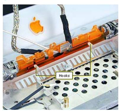
6. Move the display straight back to clear the two hooks near the center of the clutch.
