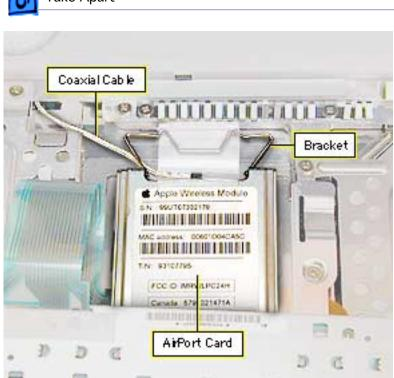
6 Flip up the wire bracket, and remove the installed AirPort Card from its connector. Disconnect the AirPort antenna coaxial cable.
