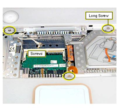
trackpad cable connector, only enough to release the trackpad cable. Do not remove the connector.
