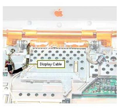
and deroute the cable from the Logic board EMI shield.
