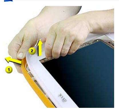
7. Work your hands around each side, separating the bezel from the display housing. At the top corners, pull the plastic of the display housing out while pulling up on the bezel.
