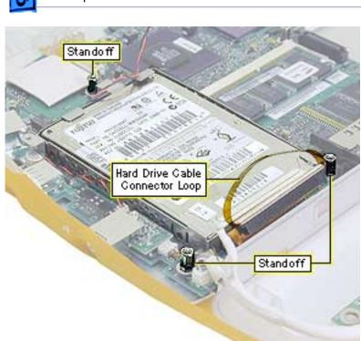
**Important:** Pull straight up to prevent bending pins on the logic board.
